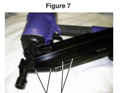
Probe in these areas with a screwdriver to release jammed nails.
